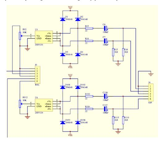
The DRV134 balanced line driver and the SSM2142P before it can both be damaged by an external voltage source such as phantom power being shoved up the output. The Hux Universal Balancing amplifier uses several lines of defence to ensure that phantom power can not cause any damage or impede the normal operation of the unit in any way.
