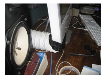
The air intake for the original version of the G5 iMac is on the left underside of the monitor. The end of the flexiduct is simply gaffa taped over the internal fan air intake. Block all air holes as best you can but don't be concerned about a little bit of air escaping out the under side of the monitor.
