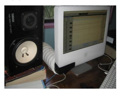
The new external fan will now gently force feed air into the iMac. You will find that the internal iMac fan will cycle down to its lowest setting and will be barely audible. The external fan can be simply left on the floor or moved into another room if you want everything to be ultra quiet.
