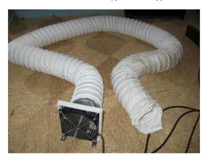
Above shows the hardware to be used in the cooling mod. The main ingredient is a 3 metre length of 100mm air duct (normally used to slurp humid air out of bathrooms), an end bracket for the duct, a slow or medium speed fan (blowing into the duct), a power cord for the fan, a fan finger guard and a couple of angle brackets for feet.
