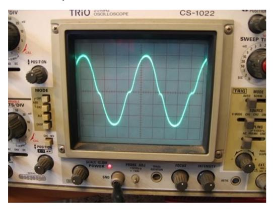
The above shows a guitar amplifier where the output valves are over-biased. As mentioned earlier, the higher the bias in a valve amp the less that the output valves can conduct. The amplifier as shown above has a lot of crossover distortion (the point where one valve hands off to the other), it is running "cold" and will not sound very good (it will be dull and lifeless).
