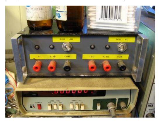
The above shows my guitar amp dummy load, this box contains 4 x 8 ohm 100 watt non inductive resistors, in Australia these can be purchased from Wagner Electronic Services in Sydney (most audio repair people have an account with WES). Each of the two channels in the box can be switched for 4, 8 and 16 ohms.
