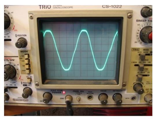
The above shows the same amplifier and the same correct bias point. The level has now been increased to push the amplifier harder into clipping and the crossover kink is now more obvious. As mentioned, the crossover kink should pretty much disappear when the level is dropped below clipping when the correct bias point has been set.
