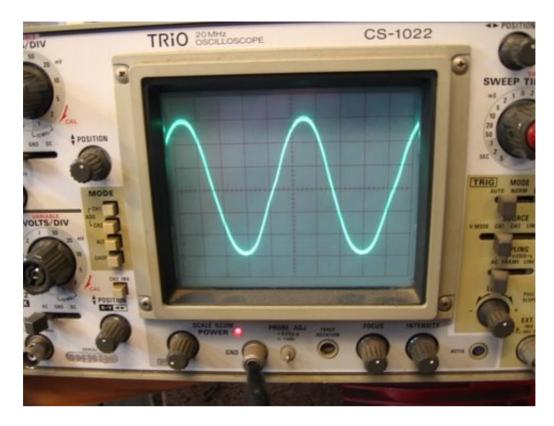
The above image shows the same amplifier with correct bias. The output is shown just under the clipping point, you can just see a small kink in the sine wave at the crossover point (the mid point between the +ve and -ve peaks). This kink should disappear when the output level is dropped away from the clipping point. This is the sweet spot where good tone occurs. There is no need to eliminate the kink completely but it should only be noticeable just on or just over the edge of clipping.
