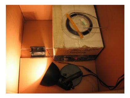
Above shows the inside of the **tape bake box**. The lamp is a standard bedlamp fitted with a 100 watt bulb. A 12 volt 80mm fan (in this case a Papst model 8312) is sitting on a section of foam (to absorb vibration) and is blowing air away from the lamp and
