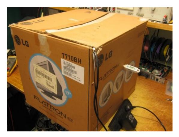
The box "as is" has a little trouble getting to 130 degrees F on a cold day. I experimented with taping up the air holes with gaffa tape etc but found that the best approach was to simply place a folded beach towel over the top of the box. The idea is to drive the moisture out of the tape, therefore there is no point sealing the box as you will trap the moisture, a beach towel helps the box to reach its desired temperature and still allows the moisture to escape.
