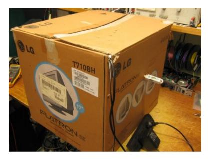
The photo above shows the **tape bake box** concept. I used the old cardboard box that my last VGA computer monitor came in, it is a perfect size.
